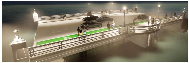
End Pylon Option 6 with Custom Luminaires and Forms+Surfaces LED Post-Top Luminaire on Mid-Bridge Pilasters and Under Top Rail Lighting AVENUE BRIDGES PROJECT
