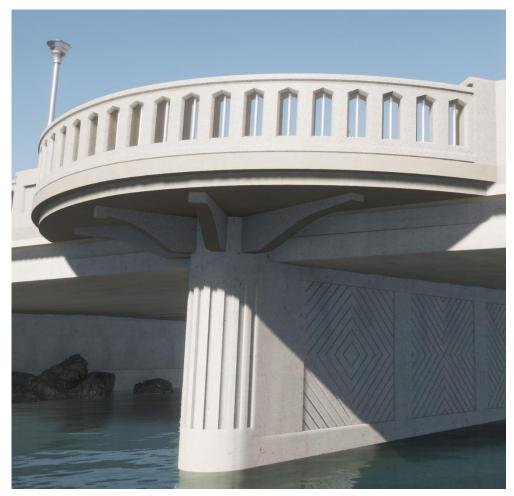
Option 1 - Overlook with Texas DOT Concrete Bridge Rail/Parapet, Brackets and Center Pier Treatment
