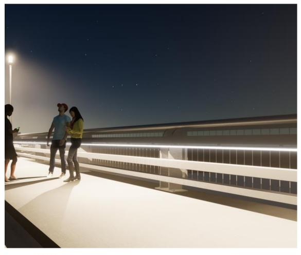
Bridge Rail Option 2 with Metal Vehicular Bridge Rail with Metal Pedestrian Fence, Forms+Surfaces LED Post-Top Luminaire on Mid-Bridge Pilasters and Under Top Rail Lighting
