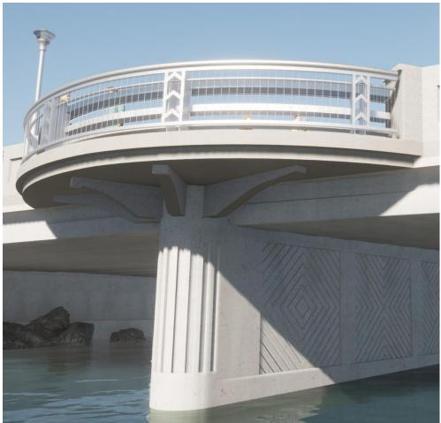
Option 2 - Overlook with Metal Vehicular Bridge Rail with Metal Pedestrian Fence, Brackets and Center Pier Treatment
