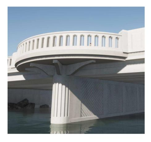
Option 1 - Overlook with Texas DOT Concrete Bridge Rail/Parapet/Overlook, Brackets and Center Pier Treatment
