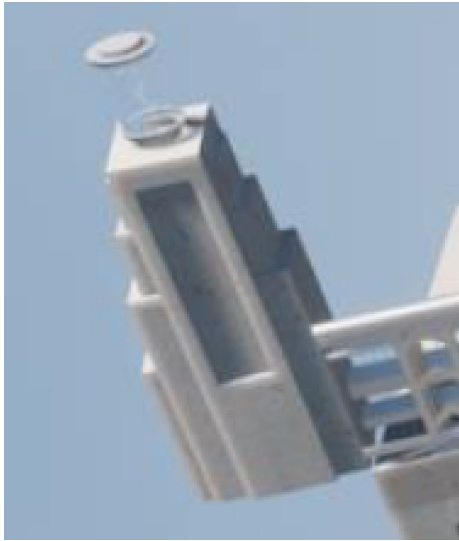
Group A: Tall End Pylon (3'-4" W x 2'-0"D x 5.0' H)
