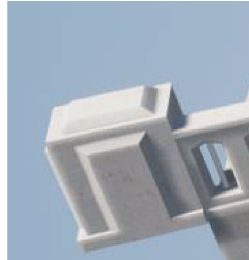
Group B: Short End Pylon (3'-8" W x 2'-6"D x 4'-6"H)
